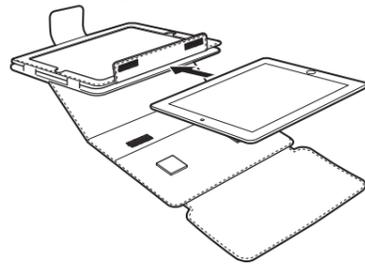
**3 Stand the iPad2 storage compartment and adjust the surface fastener.**
