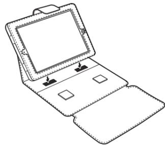
**4 Set the keyboard into the keyboard storage compartment and type from this product.**
